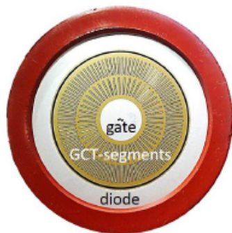
Fig. 1. The top view of 38 mm, 4.5 kV conventional RC-IGCT.
